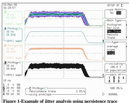
figure 1-Example of litter analysis using persistence trace functions for showing average, standard deviation, and range of the noise on a pulse waveform
